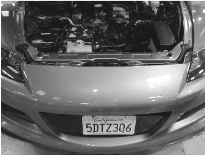
AB) Remove bumper and set aside.
