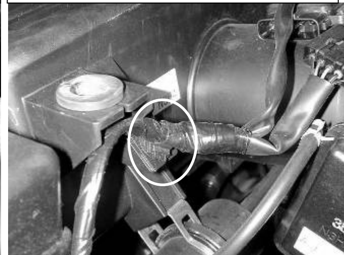
l) Remove wire tie from the air box.
