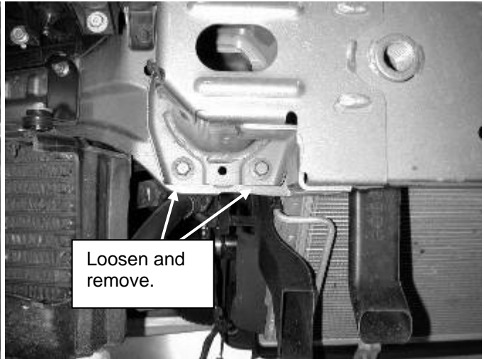
AH) Loosen and remove lower two mounting bolts.
