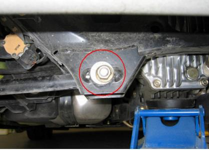
Step 12: Use a sharpie or other implement to mark the location of the alignment cam (the flat washer with marks on it circled in red) relative to the bracket. When reassembling this part you want to line these marks back up.
