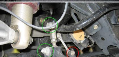
**Step 6:** Use a 10mm socket to unbolt the head light leveler arm circled in red. This is only on the left side of the car.
