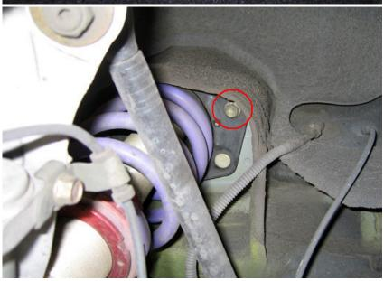
**Step 10:** Use a 12mm socket to remove the bolt circled in red. Don't be alarmed when the entire shock assembly drops a little after this bolt is removed.
