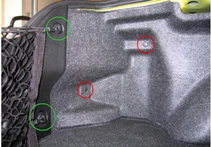
**Step 2:** Use a philips and flathead screwdriver to remove the two plastic fasteners circled in red.
