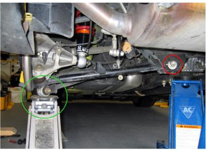
and then another black rubber part (again tapering towards the shock tower), flat washer and lock nut. Use an impact wrench to tighten the lock nut to the same depth measured in Step 17.
