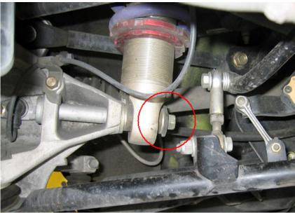
**Step 11:** Use a 17mm socket to remove the bolt circled in red.
