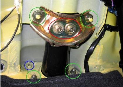
**Step 8:** Use a 14mm socket to remove the two bolts circled in red.
