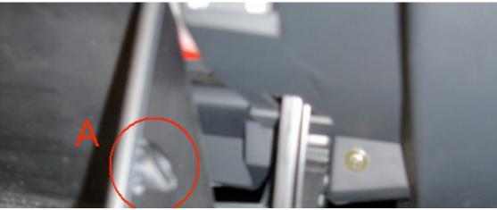
Step 1: Open the glove box. Squeeze the sides of the glove box together so the ears on each side (Circle A) clear the retaining stop.
