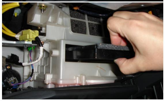
**Step 5:** Remove the two air filters from the compartment.
