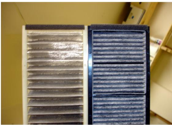
As you can see the stock cabin air filter on the left is pretty flimsy. That isn't a camera flash reflection--it's the light behind the filter shining through. By contrast the aldehyde filter on the right is much thicker. The part number is LDY3-61-J6X.
