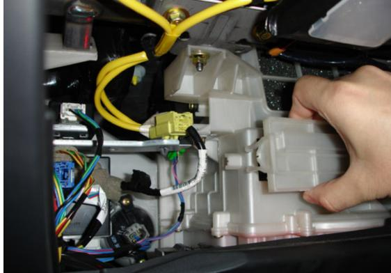
**Step 4:** Pull the air box cover straight back. It has retaining clips on either side.
