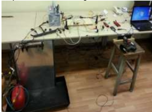
b) Setup for ignition and injection test.
