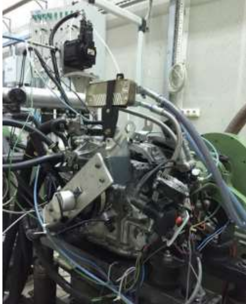
Figure 7: Drawing in the Solidworks of the single-rotor test engine consisting of essential parts (a), Single-rotor prototype test engine (b).
