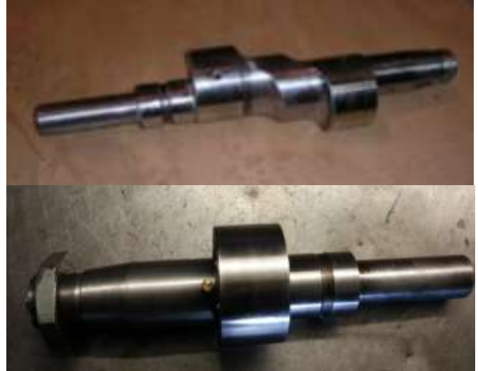
Figure 2: Conversion of two-rotor engine eccentric shaft (above) to single-rotor eccentric shaft (bottom).
