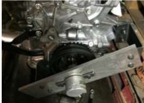
a) Encoder on the engine eccentric shaft.
