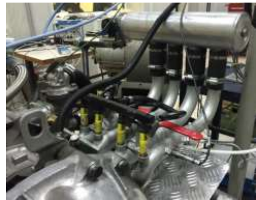
Figure 4: Intake manifold and its view (a) unassembled and (b) assembled on the engine.
